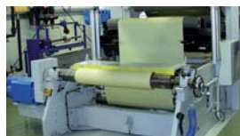
R Single Rewinder with following roller
