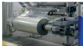
U Single Unwinder with expansion chucks
