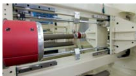
FSU Turret Unwinder with expansion chucks
