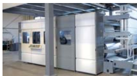
FSR Turret Rewinder with winding shaft
