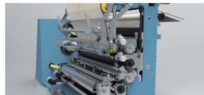
Fixed mounted coating station 800, 5 rollers for solvent-free siliconizing
