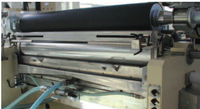
Coating station with pressurized doctor chamber blade and gravure roller. Also available as a trolley system
