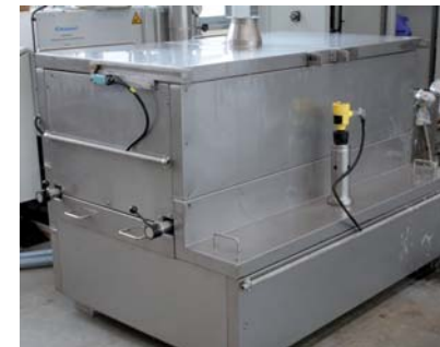
Wax melting unit PAKMELT
