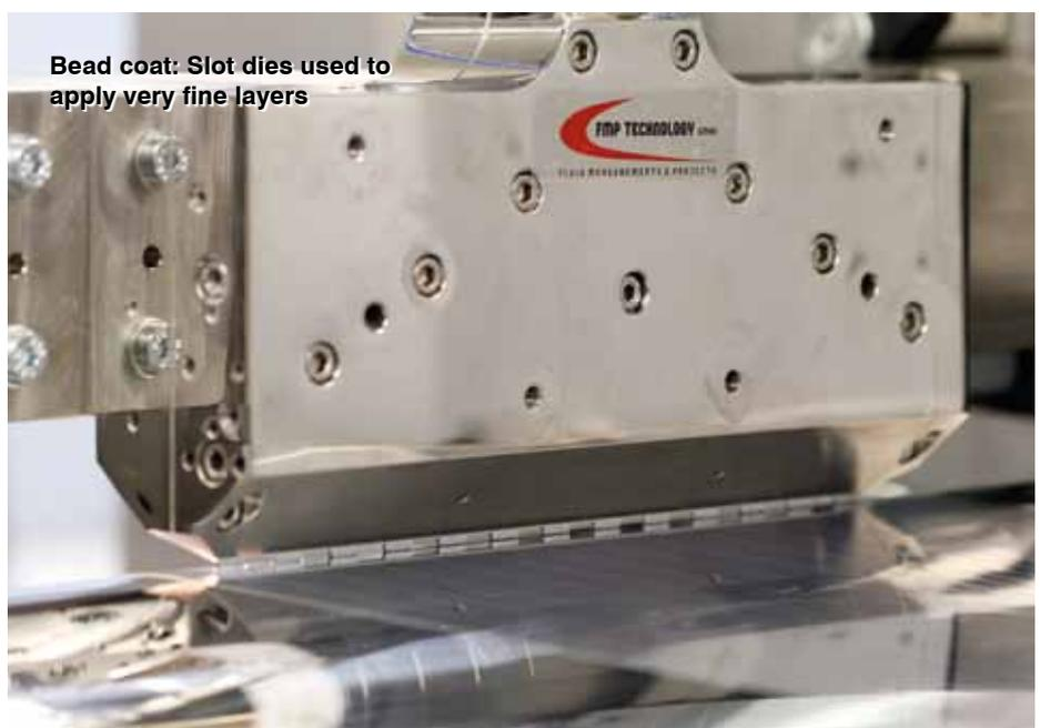
Bead coat: Slot dies used to apply very fine layers
