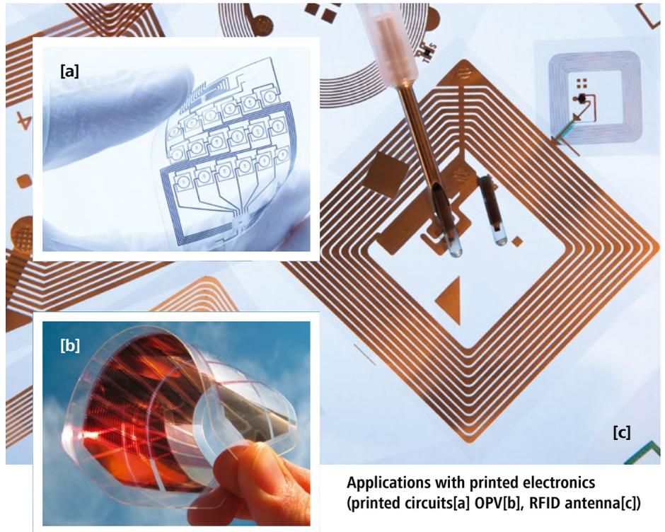
**Applications with printed electronics (printed circuits[a] OPV[b], RFID antenna[c])**
