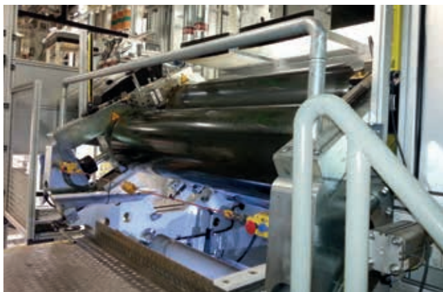
Precision coating head with four rollers allows precise control of temperature over the roller width
