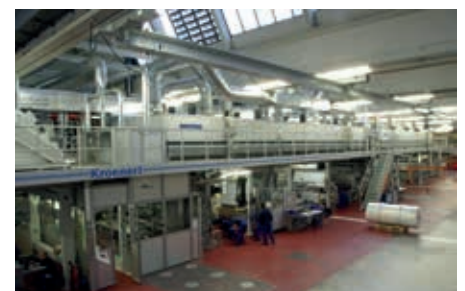
A double silicone coater at Huhtamaki (Germany, now Infiana Group)
