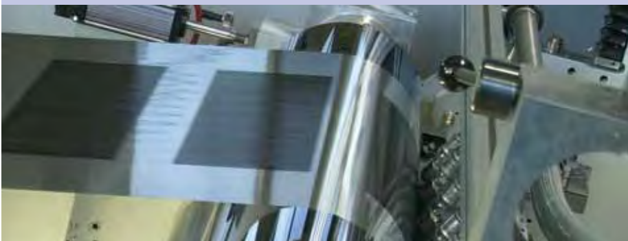
Intermittent coating for battery applications on the big RECO pilot plant
