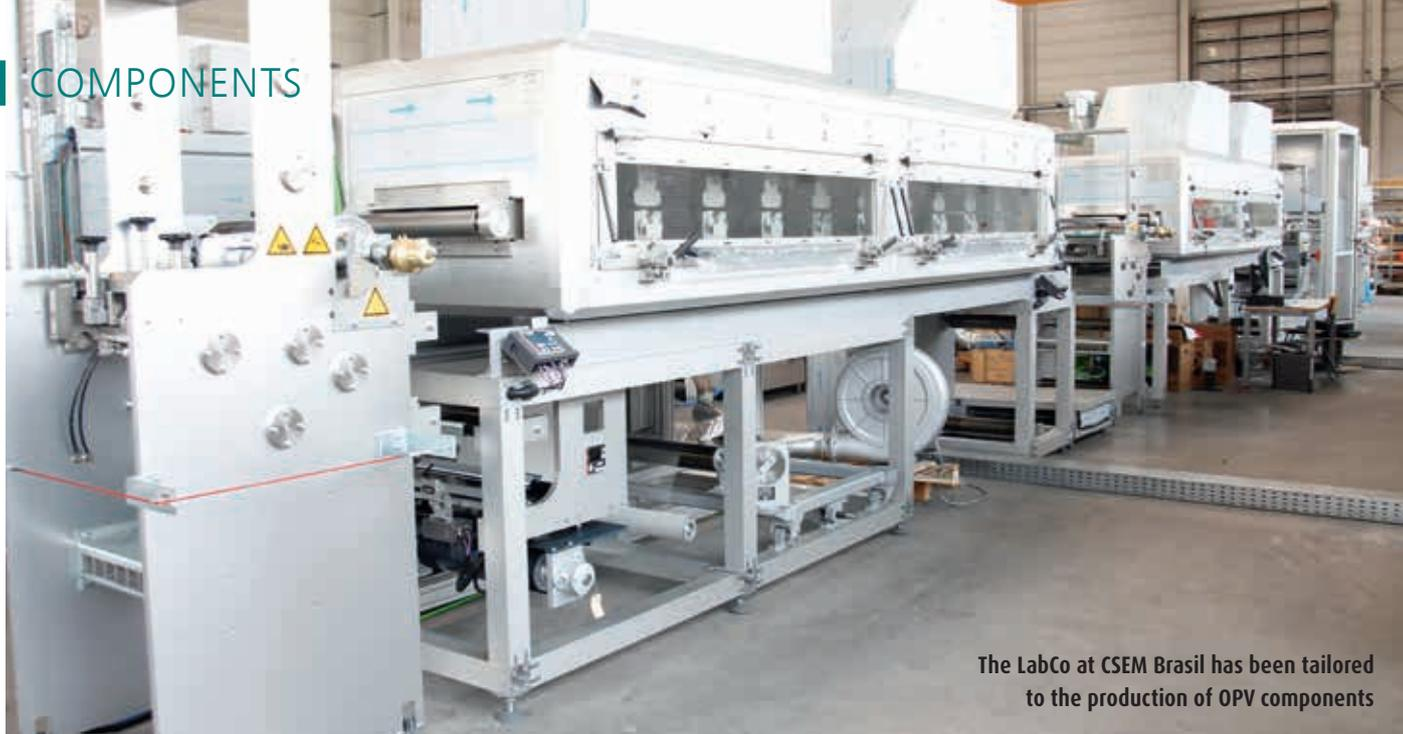
The LabCo at CSEM Brasil has been tailored to the production of OPV components
