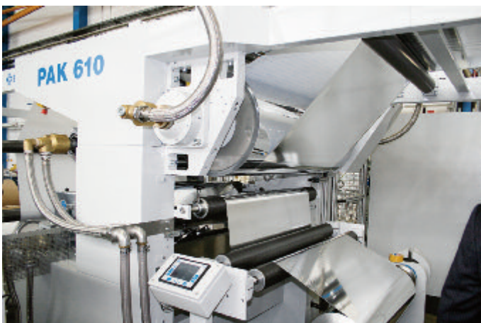
Test run of the PAK 610, demonstrating lamination of foil with paper
