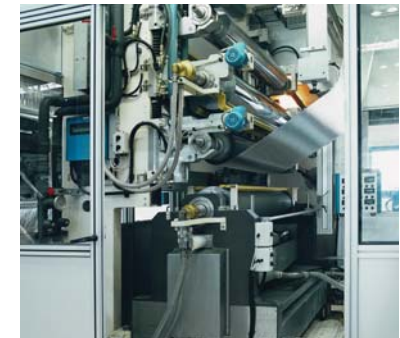
All application systems can be changed quickly because they are installed in a trolley system
