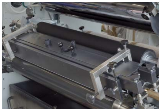
Feeding box for hotmelt coating out of the nip
