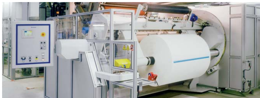
Unwinder FSU 10 AG for 2 rolls up to 1,300mm diameter
