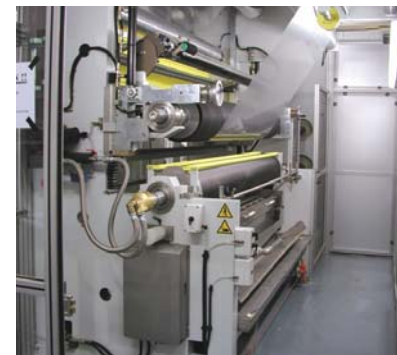
The coating system has a fixed installation in the applicator, but can be changed
