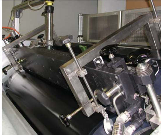
1,650-mm-wide epoxy resin applicator for applications in the aerospace, automotive and sports industries
