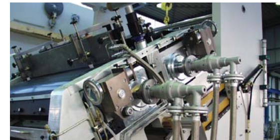
For the highest quality: Continuous cleaning of application and metering roll
