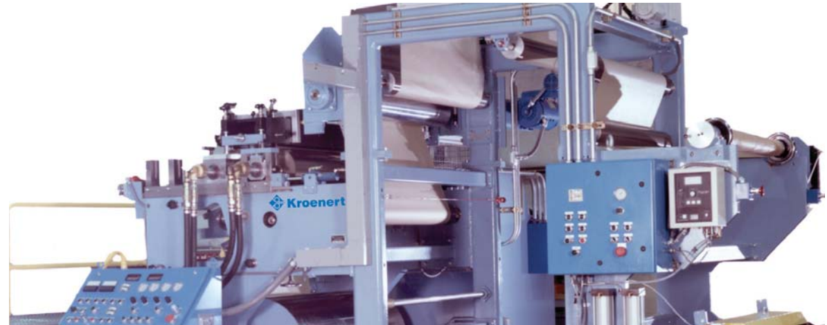
PAK 400 EP with a working speed of 150 m/min for parallel run and reverse running operation
