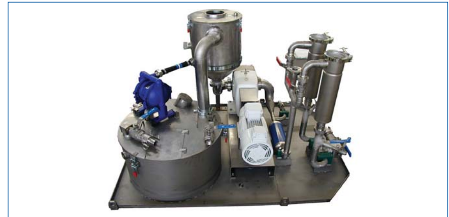
Appropriate compound circulation systems can be supplied for various rheologies and viscosities
