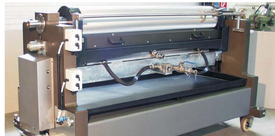
Pressure-filled chamber doctor blade with gravure roll; a repeatable chamber position is achieved by utilizing a vertical setting arrangement
