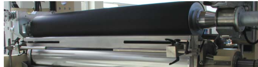
The pressure-filled chamber doctor blade combines the advantages of screen roller application with the enclosed design of a nozzle
