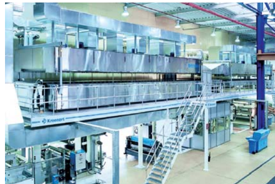
High-speed varnishing machine for 1,200 m/min.
